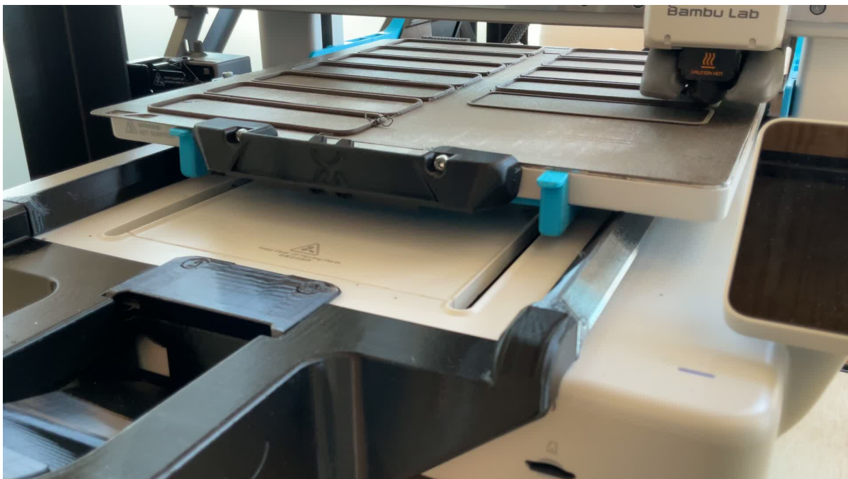
Figure 3: Several complete gasket loops printed on one build plate. The repeated geometry makes toolpath consistency and defect prevention especially important.
