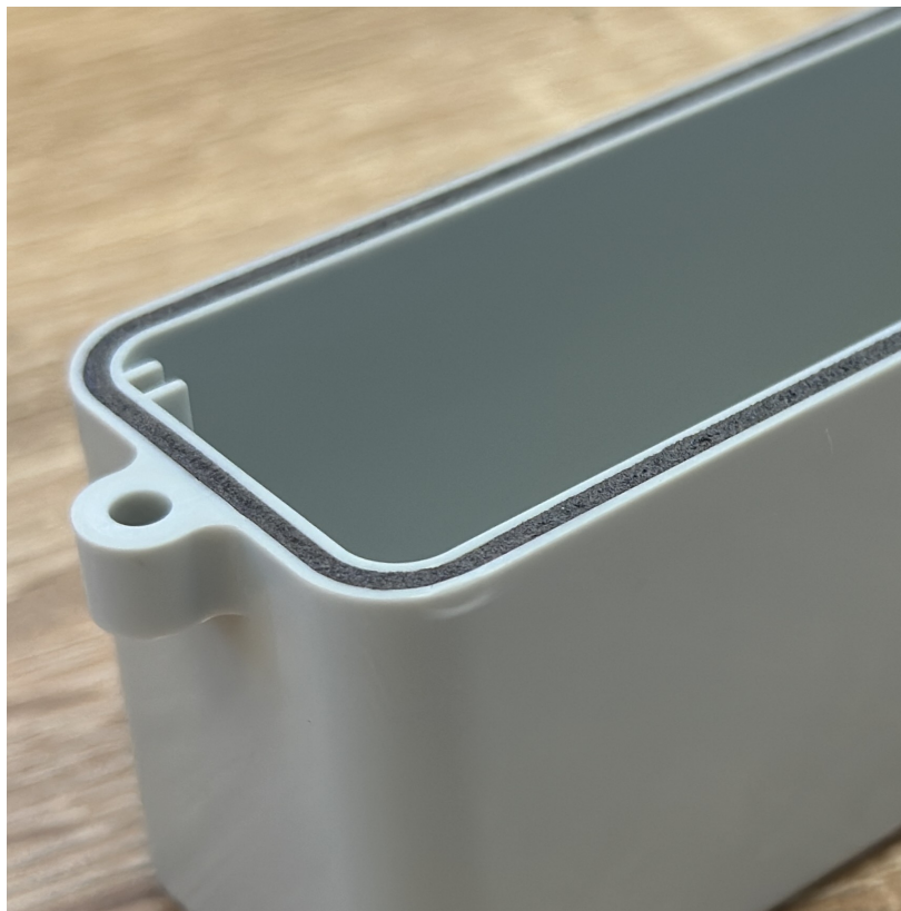
Figure 4: Installed FiberFlex Aero gasket following the enclosure groove. The foam texture allows the bead to compress and remain seated during assembly.
